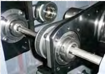
同步迴轉導套 Synchronous rotary guide bushing device
