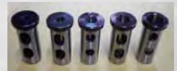
內孔套筒 (外徑 \varnothing 20 ) (I.D \varnothing 6,8,10,12,16 / O.D \varnothing 20 ) Tool holder bush
