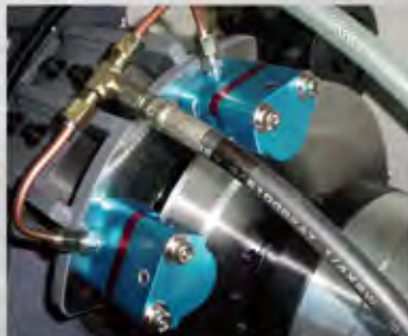
C軸功能-碟刹裝置 C-axis function (Disc brake device)
