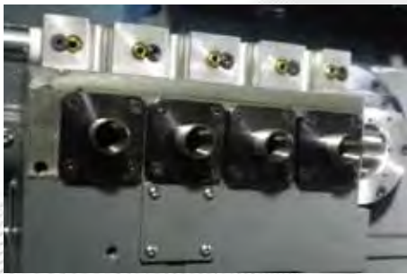
副主軸端面4軸動力刀具裝置 End side 4-shaft live tooling device for sub-spindle
